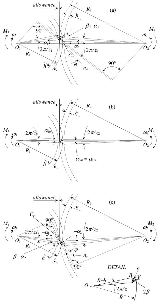
Fig. 2. Scheme of tooth coupling.  $z_2/z_1 = 2$ ,  $\beta = 30^\circ$ .
