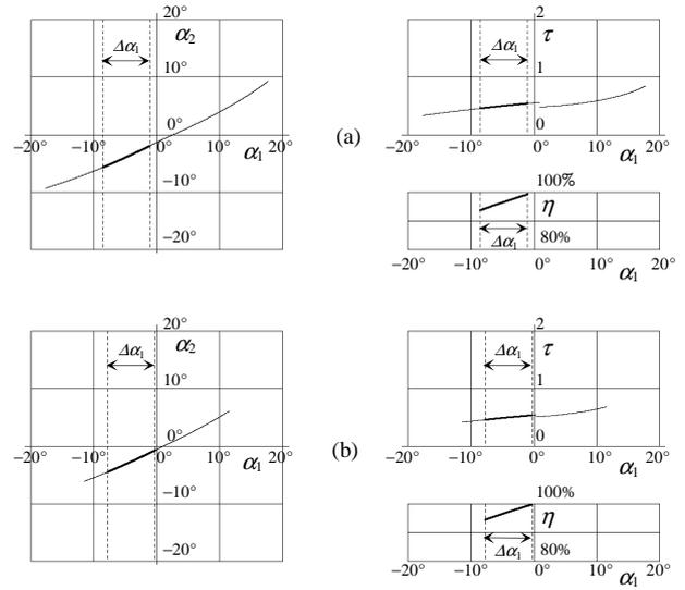
Fig. 3 a, b. Secondary rotation  $\alpha_2$ , speed ratio  $\tau$  and sliding efficiency  $\eta$ , in dependence on the driver gearwheel rotation  $\alpha_1$ .  $\Delta\alpha_1 = 360^\circ/z_1$ .
