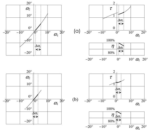
Fig. 4 a, b. Secondary rotation  $\alpha_2$ , speed ratio  $\tau$  and sliding efficiency  $\eta$ , in dependence on the driver gearwheel rotation  $\alpha_1$ .  $\Delta\alpha_1 = 360^\circ/z_1$ .
